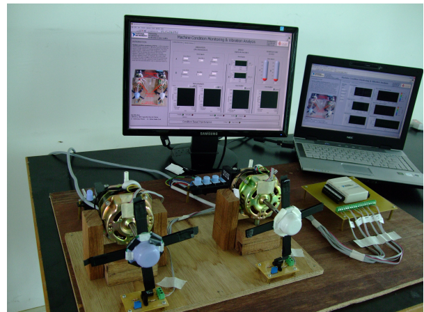
Fig.9 Implementation of the Sensing setup and DAQ unit
