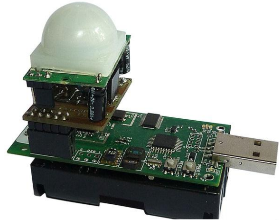
Figure 3: TelosB mote equipped with boost converter and PIR sensor module
