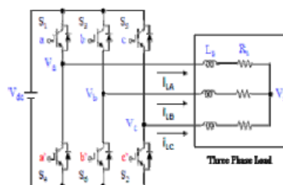
Figure.1 Three-Phase two level voltage source inverters
