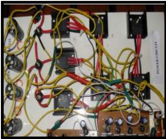
Fig.9. Fabricated single-phase SNLI circuit.
