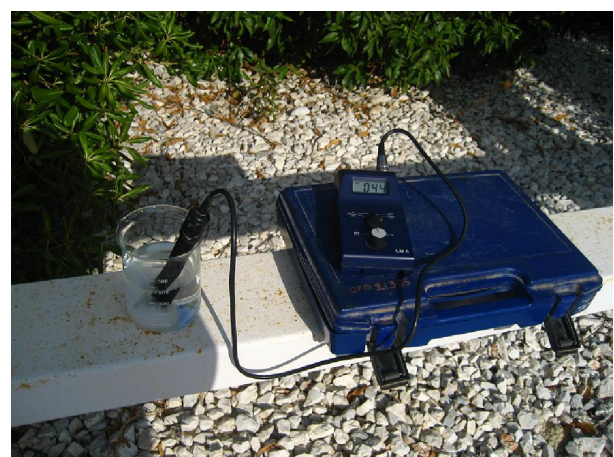
Fig. 6 Measuring ESDD on site
