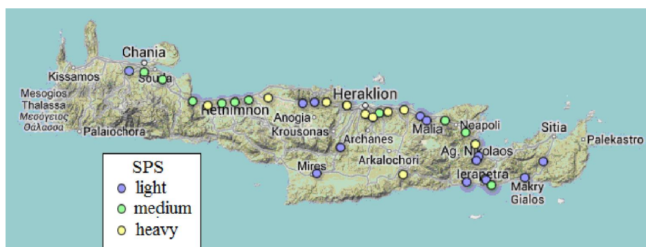
Fig. 7 Site Pollution Severity using the limits proposed by IEEE
