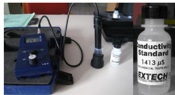
Fig. 5 Calibration and accuracy verification using a solution of standard conductivity
